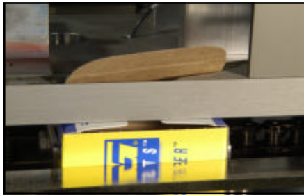
Carton closing on the TC 50 can be done via straight or reverse tuck (shown above), or hot melt glue.
