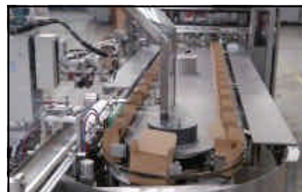
The Victory 100 carton track provides opportunities for robotic integration, while also allowing for hand loading or other auto load components.
