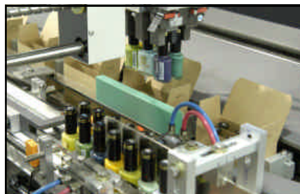
Tisma's end tooling, attached to robotic unit, places bottles in 2 x3 pattern into the carton.
