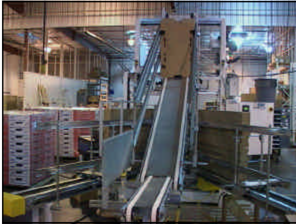
The above photo shows SWF’s BF 600V forming the Kisch Bliss, with an attached Ergo Hopper and extended end panel hoppers.
