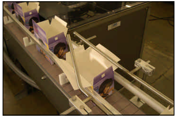
The Victory 100 discharges newly formed cartons and opens major flaps prior to robotic loading. Carton sealing occurs downstream, inline, after loading.
